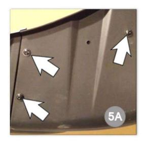
Mount the bumper on the truck by starting all bolts and then tighten. You can hold the bumper in place by using a jack underneath it if you choose to do so. You will use the top and bottom holes on the face-mount. You will not use the center hole. (Picture 6A) You will also insert and tighten the two bolts for the bumper end mount support, located above the fog light. You will repeat this step for the other bumper end.
