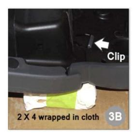
Make sure the clips are completely fastened together. The Image on the right shows you what it will look like when the clip is properly fastened together. (Picture 3C) Make sure this is the same for all three clips for this side of the bumper. You will do the same thing for the other side of the bumper as well.
