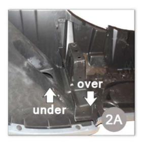
Once you have the center bumper piece and bumper end overlapping, locate the three clips that will secure the two pieces together. (Picture 3A)
