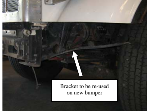
Step 2: Remove (& save) all mounting brackets
