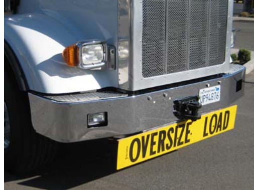
Step 4: Re-install all brackets onto bumper
