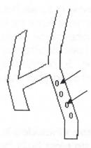
CAUTION: When hood is closed the snubber brackets on the hood must bottom out on cab bracket or the hood will not ride securely.
