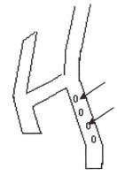
CAUTION: When hood is closed the snubber brackets on the hood must bottom out on cab bracket or the hood will not ride securely.
