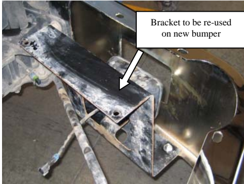
Step 1: Remove Factory Bumper
