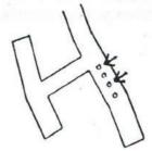
CAUTION: When hood is closed the snubber brackets on the hood must bottom out on cab bracket or the hood will not ride securely.
