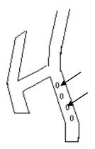
CAUTION: When hood is closed the snubber brackets on the hood must bottom out on cab bracket or the hood will not ride securely.
