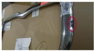
Flange cracking due to damage originating at other locations
