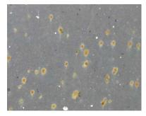
Random red spots and other visible damage to the chrome plating layer due to road debris strikes
