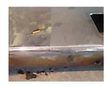
Corrosion on bottom flange of the bumper
